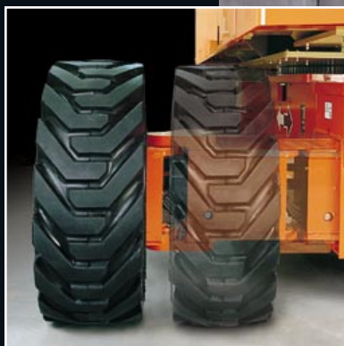
Pin-less Axle Extension for Faster Setup
